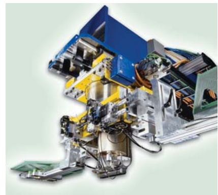
Handling system precision blanking with direct drives
